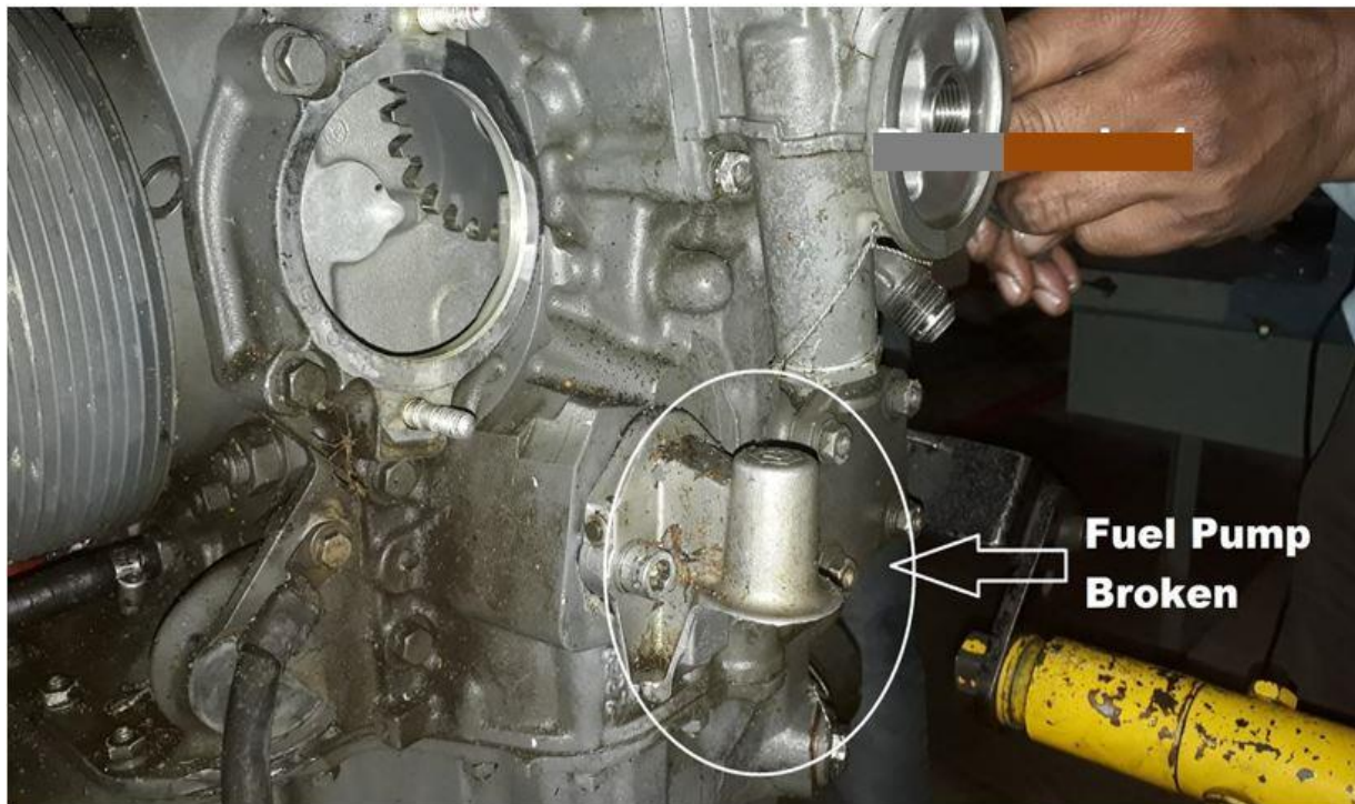
Fig: 29: Broken fuel pump
