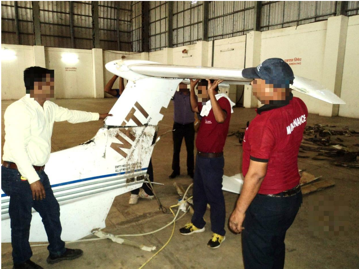
Fig 11: Wreckage of vertical stabilizer
