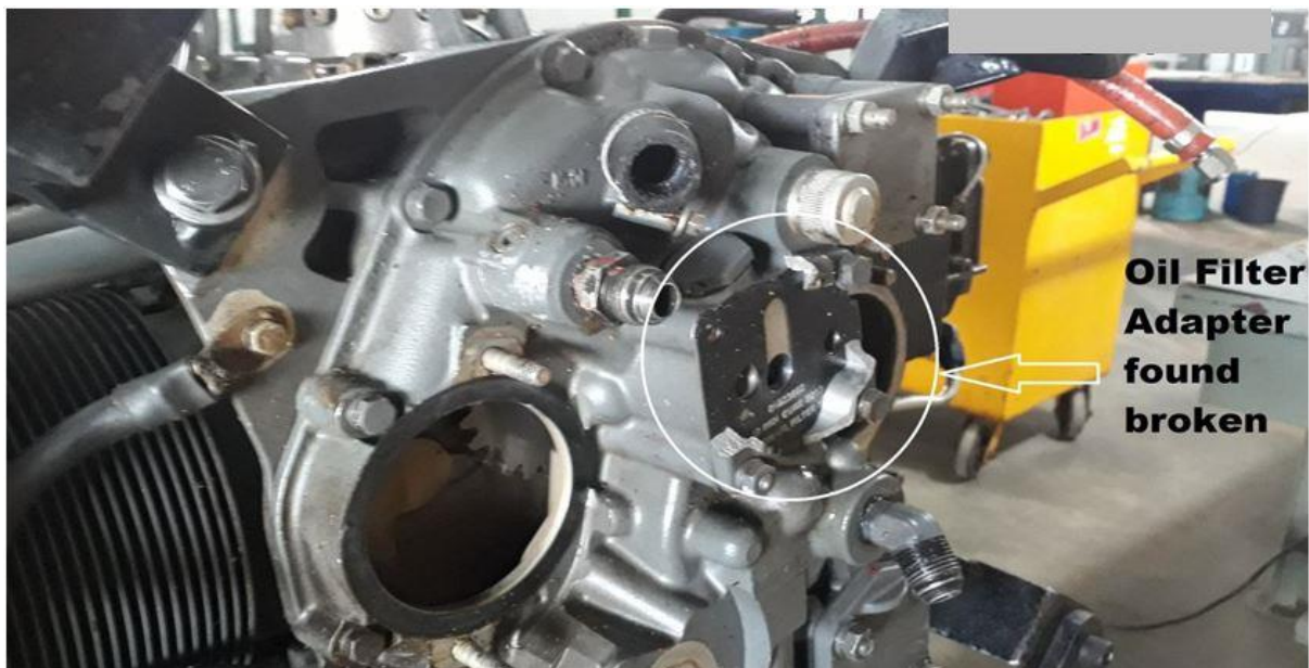
Fig: 26: Broken oil filter adapter
