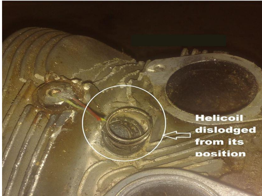
Fig:19: Dislodged Helicoil
