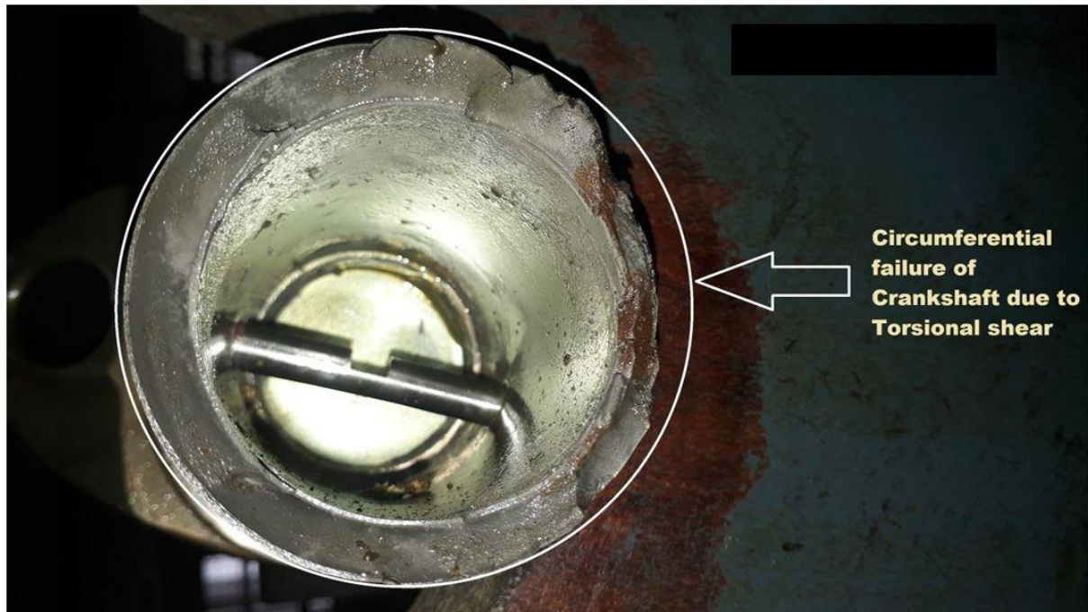
Fig: 23: Failed crankshaft
