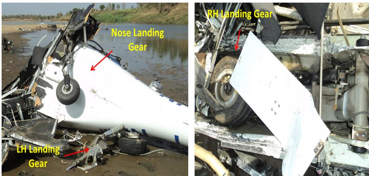
Fig 13: Landing gears at crash site
