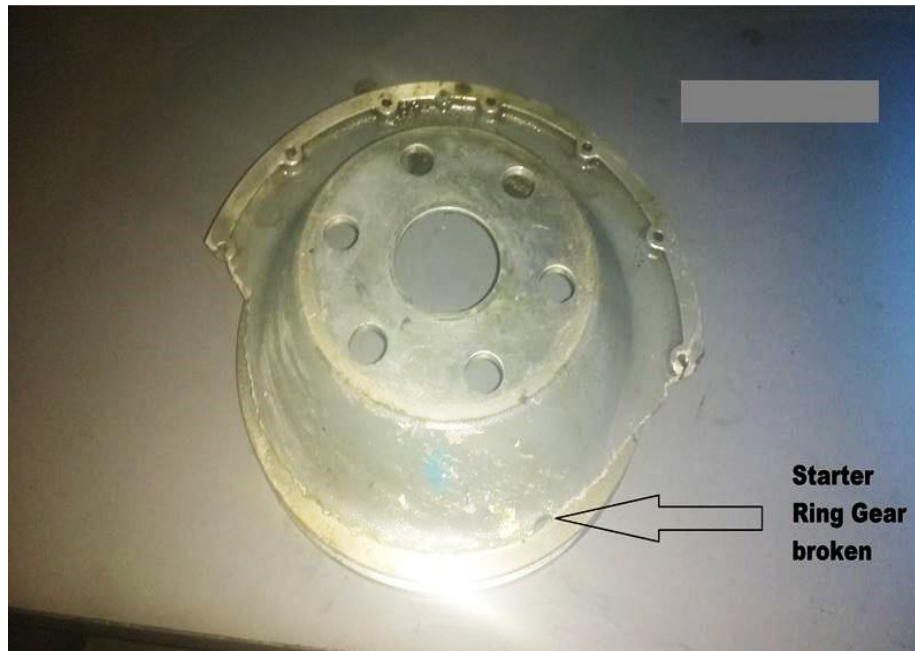
Fig: 30: Broken starter ring gear
